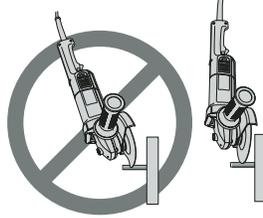
5. Remove the tool from the work surface before turning the tool off. Allow the tool to stop rotating before laying it down.
